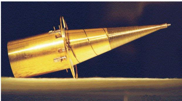
TIM's electrical substitution radiometer (ESR) has enabled SORCE to measure the solar irradiance with an improvement in precision by more than a factor of 10. **Image credit:** LASP
