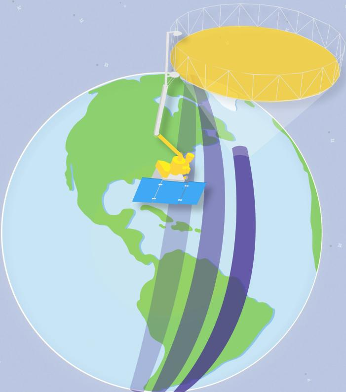
The Soil Moisture Active Passive, or SMAP, satellite is designed to image 1,000-kilometer-wide swaths of Earth from a near-polar, sun-synchronous orbit 685 kilometers above Earth's surface.
